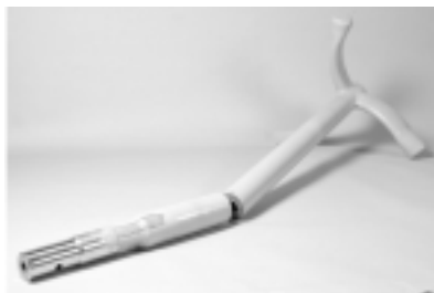
Damaged upper end removed from shaft
