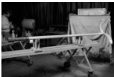
Finished agitator with repairs completed
