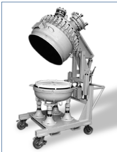
Nutsche Filter showing the glass-lined interior, filter plate assembly and hydraulic lift stand.
